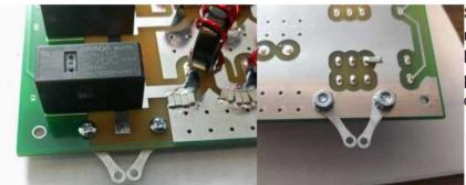
Secure two solder lugs as shown here using the 4-40 machine screws provided; leftmost photo is top side, rightmost photo shows the two locking nuts on the other side securing the lugs.
