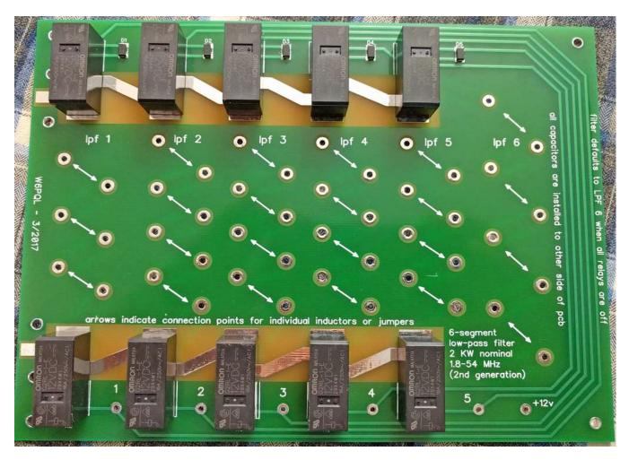
Turn the board over and install the chip capacitors. The 6m segment is on the left, 160m on the right. The photo is for the single-pallet configuration; the dual pallet will be similar.
