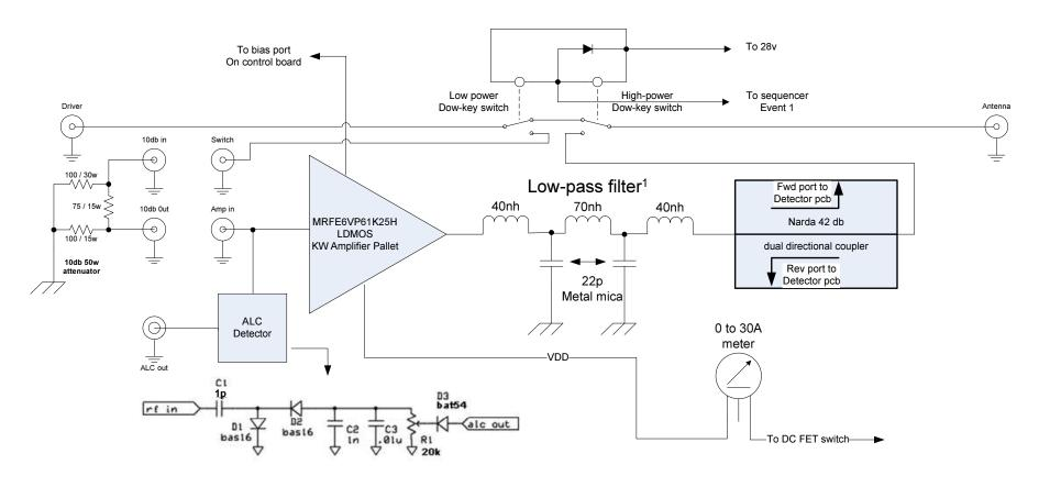
1. insertion loss < .05db @ 144 MHz. Return loss > 25db. Attenuation > 18db @ 288 MHz, and > 30 db @ 432 MHz. Inductors are 2t #14 solid, space-wound, 11/32" diameter, and 4t, 5/16 dia.
